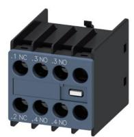
auxiliary switch, on the front, 2 NO + 1 NC, .1/.2, .3/.4, .3/.4, .-/--, current path: 1 NC, 1 NO, 1 NO, --, screw terminal, for contactors 3RT2 and contactor relays 3RH2
