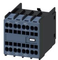
auxiliary switch, on the front, 1 NO + 2 NC, .1/.2, .1/.2, .3/.4, --/--, current path: 1 NC, 1 NC, 1 NO, --, spring-loaded terminal, for contactors 3RT2 and contactor relays 3RH2
