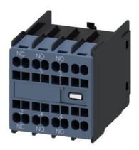
auxiliary switch, on the front, 2 NO + 1 NC, .1/.2, .3/.4, .3/.4, .-/--, current path: 1 NC, 1 NO, 1 NO, --, spring-loaded terminal, for contactors 3RT2 and contactor relays 3RH2
