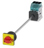
Load disconnector 3LD3, lu 63 A Main switch 3-pole Rated operating capacity at AC-23 A at 400V 22.0 kW floor mounting Basic switch with door coupling Central hole mounting 22.5mm Toggle drive red / yellow 48x48 mm
