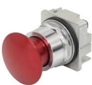
30mm Command/52, Chrome Finish Heavy Duty,Watertight/Oiltight Metal Operator, Round Push-Pull Operator Non-Illuminated Mushroom Head Cap Small 1.73" (44 mm) Metal, Anodized Red 2 Position Maintained, Pull-to-Release UL Listed, CSA Certified NEMA 1,3,3R,4,4X,12,13 & Automotive Standards
