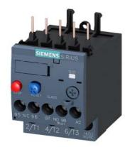
Overload relay 4.5...6.3 A Thermal For motor protection Size S00, Class 10 Contactor mounting Main circuit: Screw Auxiliary circuit: Screw Manual-Automatic-Reset
