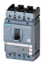
circuit breaker 3VA5 UL Frame 250 breaking capacity class M 35 kA @ 480 V 3-pole, line protection TM230, FTAM, In=200 A overload protection Ir=200 A permanently set short-circuit protection li=5...10 x In cable connection on two sides
