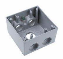
Weatherproof 2 Gang Deep Box, 5 Hole 1 37 Cu.In. with Threaded Holes, Gray (2 Holes Each End, 1 Hole in Back)
