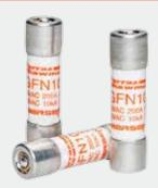
GFN midget indicating fuses are available in ratings from 1/10 through 30A. These time-delay fuses have built-in blown fuse indicators which pop out at the end of the fuse to visually indicate when the fuse has operated to open the circuit. Indicators may be used to trip a switch for remote as well as visual annunciation. (Not for Branch Circuit Protection).
