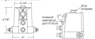
Due to yoke design, the TFM will be off center when mounted.
