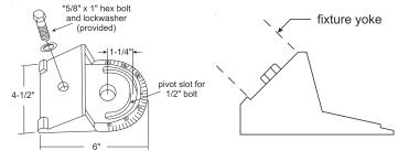
Due to yoke design, the TFM will be off center when mounted.
