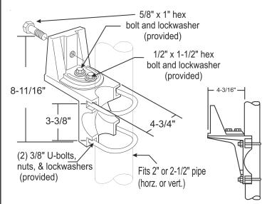
Due to yoke design, the TFM will be off center when mounted.
