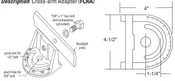
Installation: Secure the fixture yoke mount to the FCRA or FCRA45 by using the bolt and lockwasher provided. Secure the FCRA or the FCRA45 to the cross-arm with a 5/8" bolt (not provided).
