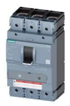
circuit breaker 3VA5 UL Frame 400 breaking capacity class C 100 kA @ 480 V 3-pole, line protection TM230, FTAM, In=400 A overload protection Ir=400 A permanently set short-circuit protection Ii=5...10 x In cable connection on two sides
