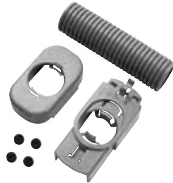
2. Place base divider (#UDBD) in the bottom of the floor box by pulling the electrical wires through the center opening. Compress the base divider (#UDBD), allowing it to slide freely down into the box. Align the base divider (#UDBD) with the desired hubs. Press the locating tab down to secure the base divider (#UDBD) into position.
