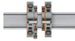
**Stepping down via push-in type jumper bar:** Commoning via open terminal side with end plate allows jumpering over two cross-section sizes for 16 mm<sup>2</sup> (6 AWG) and 10 mm<sup>2</sup> (8 AWG) and one cross-section size for 6/4/2.5 mm<sup>2</sup> (10/12/14 AWG). An example: from 16 mm<sup>2</sup> (6 AWG) to 6 mm<sup>2</sup> (10 AWG) (see illustration above) or from 10 mm<sup>2</sup> (8 AWG) to 4 mm<sup>2</sup> (12 AWG).
