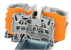
Step-down jumpers common terminal blocks of different sizes, without losing a conductor clamping point. This can be beneficial on long conductor runs where voltage drop can be a problem. A large conductor can be easily connected to smaller conductors at the distribution point. Commoning may be made in either direction using the special thin end plate to cover the open side. Additional through terminal blocks having a smaller cross-section may be commoned using push-in type jumper bars.
