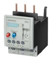
Overload relay 22...32 A For motor protection Size S2, Class 10 Contactor mounting Main circuit: Screw terminal Auxiliary circuit: Screw terminal Manual-Automatic-Reset !!! Phased-out product !!! Successor is SIRIUS 3RU2 Preferred successor type is >>3RU2136-4EB0<<
