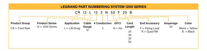
WWW.LEGRAND.US/PASSANDSEYMOUR \_\_\_\_\_\_ CABLE REELS \_\_\_\_\_
