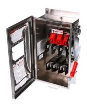
Siemens Low Voltage Circuit Protection Heavy Duty Safety Switches. Type: ENCLOSED, SAFETY SWITCH Std: UL V. Rating: 600V A. Rating: 200A No. Of Poles: 3P F. Rating: 60Hz Action: SINGLE THROW Material: SS Enclosure: TYPE 4X. 2-3 point mounting holes. Insulation: YES O. Cycles: 8000 O. Temperature: (-20F-120F) AMBIENT TEMPERATURE Environmental Conditions: INDUSTRIAL CORROSIVE RESISTANCE
