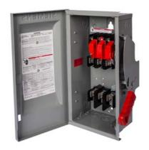
Siemens Low Voltage Circuit Protection Heavy Duty Safety Switches. Type: ENCLOSED, SAFETY SWITCH Std: UL V. Rating: 600V A. Rating: 200A No. Of Poles: 3P F. Rating: 60Hz Action: SINGLE THROW Material: 304SS Enclosure: TYPE 12. 2-3 point mounting holes. Insulation: YES O. Cycles: 8000 O. Temperature: (-20F-120F) AMBIENT TEMPERATURE Environmental Conditions: INDUSTRIAL
