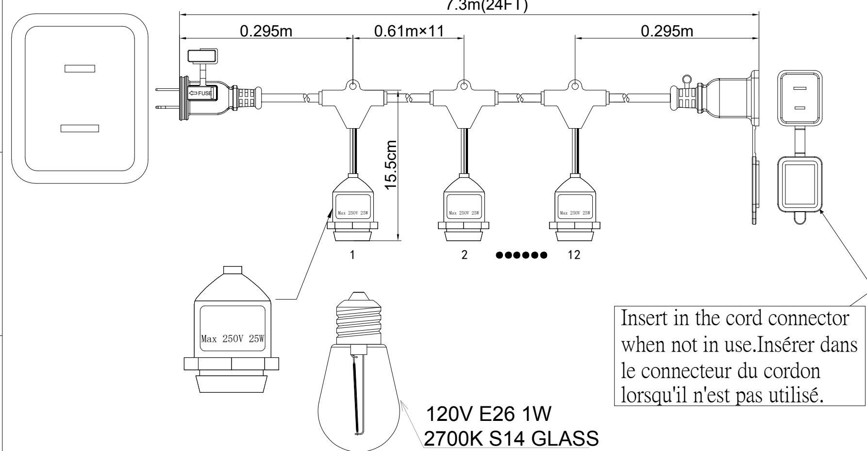
cable: SJTW 2×0.824mm<sup>2</sup> (18AWG)  $\phi$ 7.2mm black
