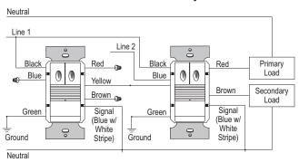
Signal wire connects to neutral. Signal wire can connect to ground in replacement or retrofit application
