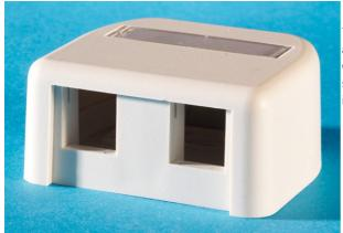
TechChoice surface mount boxes accept 2 rear loading keystione jacks & modules and provides easy snap-on covers and snap-in label fields. Boxes are supplied with screws and double-sided adhesive tape for mounting onto almost any surface. The 1 and 2 port versions are rated UL2043 and are suitable for installation in air handling spaces (ie plenum spaces).
