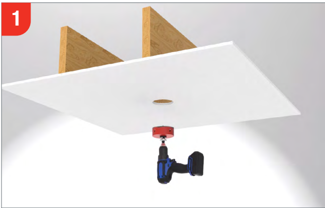
1 Create Opening with Hole Saw
