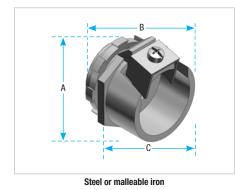
Easy to install with double grip saddle. These fittings are completely salvageable. The 3/8 in. and 1/2 in. sizes are made of formed steel which produce a uniform high quality and a smooth throat that protects conductor insulation. 3/4 in. and larger size are malleable iron
