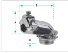
The angle clip gives secure mechanical grip that tightens under tension or vibration. Throat is long enough to install in cast housing knockouts. The 3/8 in. and 1/2 in. sizes are of steel construction. The 3/4 in. and larger sizes are malleable iron.
