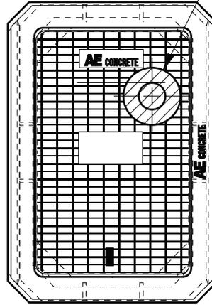
**Cast Iron Cover c/w Hole for Remote Reader**
